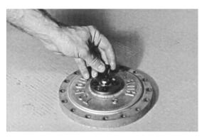
9. Using a torque wrench, apply 2.95 to 3.69 ft. lbs. (4 to 5 Nm) of torque to both bolts (6C).
