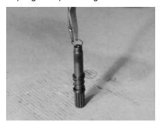
With large splined end down, place input shaft subassembly (7) into spindle (1A).
