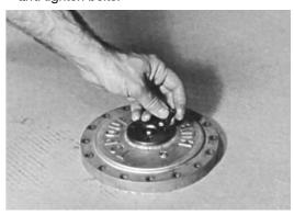
6. Using a torque wrench, apply 2.95 to 3.69 ft. lbs. (4 to 5 Nm) of torque to both bolts (6C).
