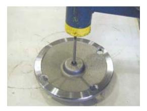
21. Install preassembled Cover (8) into Ring Gear (22).
