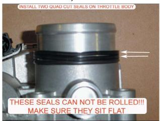
Attach mixer and throttle body together. The two parts do not bolt together; they will be secured when you mount it on the intake. Notice the orientation of the air inlet and throttle body cover.
