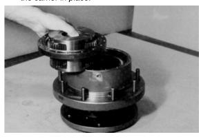
14. With the internal splines facing up (counterbore end facing down), place input gear (8) into mesh with carrier sub-assembly (3).
