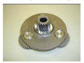
**NOTE:** Heat Supporting Ring (6) to approximately 189.5° F (70° C) in a heating furnace.
