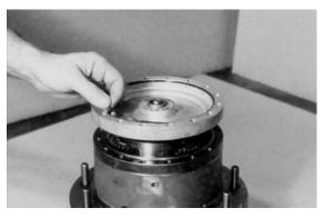
17. Place cover sub-assembly (6) onto ring gear (4), aligning the pipe plug holes according to the alignment prior to disassembly.
