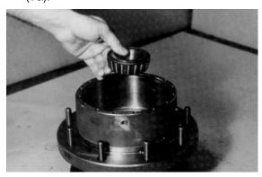
9. Place spacer (1H) onto spindle (1A) in hub (1G).
