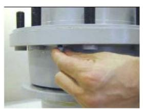
16. Install completely pre-assembled 1<sup>st</sup> planet stage into the gear drive.
