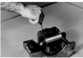
9. Drive roll pin (3G) down into the aligned roll pin holes in carrier housing (3A) and planet shaft (3E).
