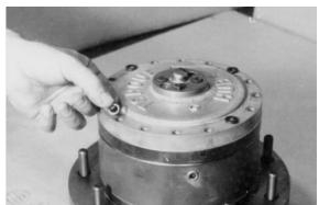
19. Place shoulder bolts (13) into the four shoulder bolt holes in cover (6) and tighten by hand.
