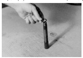
Place one spring (7C) onto the smooth end of input shaft (7A).
