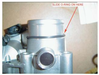
Install the two quad seals. Install one seal at a time to ensure the seal does not roll. The seal must sit flat on the throttle body.
