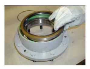
7. Install preassembled supporting ring onto Spindle (34).
