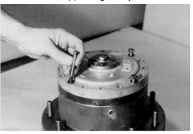
20. Place the remaining 12 flatwashers (16) onto the remaining bolt holes in cover (6).
