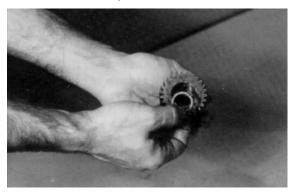
Line the remaining half of cluster gear (3F) with 16 needle rollers.
