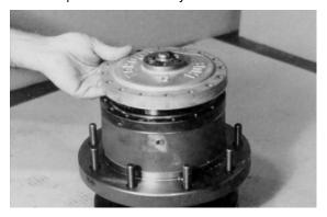
18. Place four flatwashers (16) on top of the bolt holes in the cover sub-assembly.
