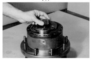
Oil all exposed surfaces inside the hub (1G). Place thrust washer (11) into the counterbore in top of the carrier.
