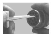
Figure 6-16. HD/HDP Contact Removal
