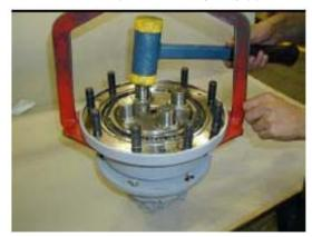
13. Remove Radial Shaft Seal Ring (17).
