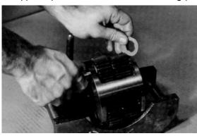
Use an alignment punch or similar tool to align the roll pin holes in carrier housing (3A) and planet shaft (3E).
