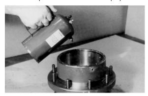
3. Place internal gear (2) into hub (1G) so that its internal splines mesh with the external splines of spindle (1A). Oil internal gear (2).
