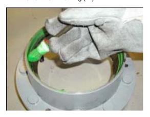
Insert the bottom part of the double Tapered Roller Bearing (11).
