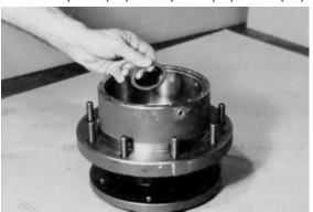
**NOTE:** Make sure the retaining ring is securely seated in the groove.
