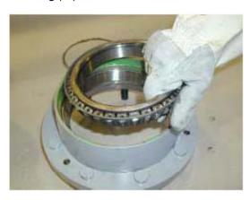
6. Insert radial Shaft Seal Ring (17) into Supporting Ring (6) and fill mounting space between sealing lips with roller bearing grease.
