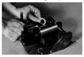
6. Following the thrust washer, place the cluster gear (3F), large end toward roll pin hole in carrier housing, onto the planet shaft (3E).
