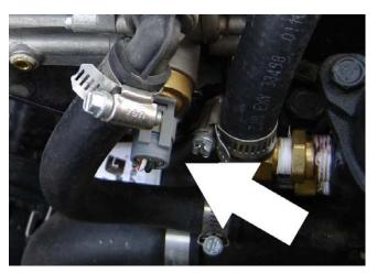
Remove the retainer clip for the LPG fuel temperature sensor and remove the sensor from the regulator body.
