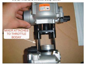
4. Place gasket on intake manifold and attach mixer/ throttle assembly to manifold.
