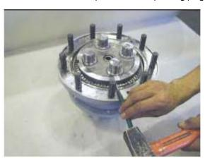
12. Insert a new greased O-Ring (16) into the o-ring groove of the Supporting Ring (6).
