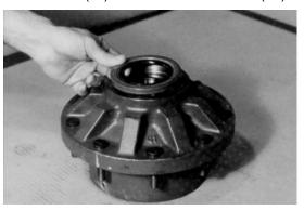
Oil spindle, then lower hub (1G), small end down, onto spindle (1A).
