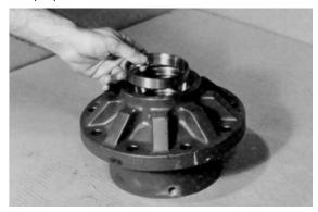
2. Press the nine studs (1N) into the stud holes in hub (1G).
