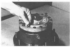
21. Place the 12 bolts into the remaining bolt holes in cover (6) and tighten.
