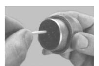
Figure 6-14. HD/HDP Contact Installation
