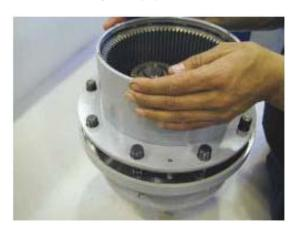
15. Install the ring gear hex head bolts. Tighten bolts to proper torque of 15.5 lb-ft (21 Nm).
