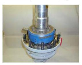
After proper bearing setting is completed, hammer ball with suitable punch, 1.1 - 1.3mm into the spindle thread. Retain ball in position with expanding plug.
