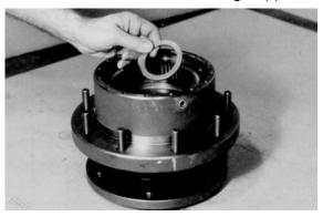
5. Stand input shaft (7A) on its splined end. Place one spacer (7D) onto the smooth end of input shaft (7A).
