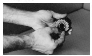
Set carrier housing (3A) sideways on a table. Insert a
