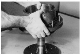
8. Press bearing cone (1F) onto spindle (1A) in hub (1G).
