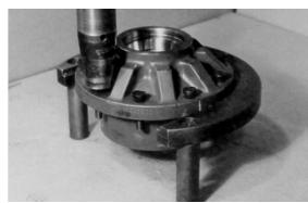
Apply a light coat of "Never-Seize" to two pipe plugs (1J) and tighten them into the two pipe plug holes in the side of the hub (1G).
