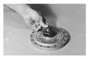
8. Place the two remaining bolts (6C) into the bolt holes in the disconnect cap (6D), and tighten the bolts.
