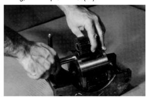
7. Following the cluster gear, place one more thrust washer (3B) onto planet shaft (3E) through the opposite planet shaft hole in carrier housing (3A).
